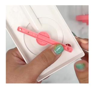
5. Place the screw through the second hole from the other end of the lever and tighten securely with a Phillips head screwdriver. Be careful to not overtighten, as this can strip the plastic. When assembled properly, pressing the spring-loaded drain button should cause the drain stopper to open slightly.
