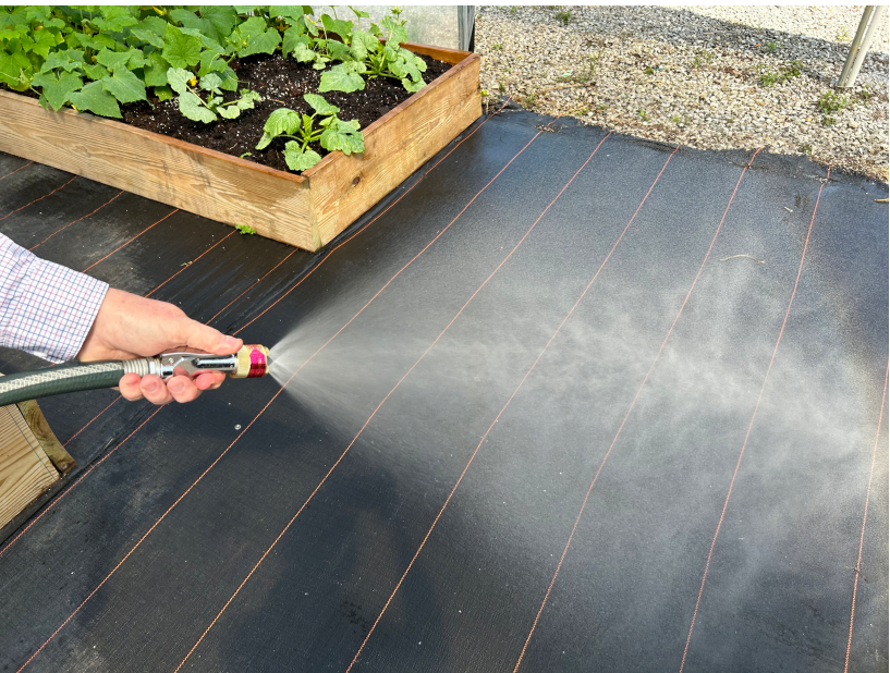
Violet Nozzle - Fine Volume - 1 GPM
