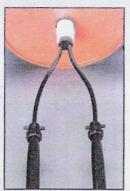
Insert large end of each barb into one end of each piece of drip tape; tighten collars.
