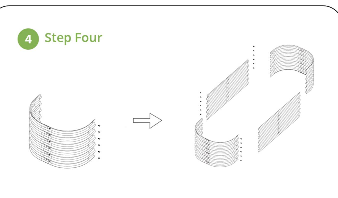
After straight panels are assembled, attach corner panels with straight panels using the same method. Make sure corner panels are attached outside of the straight panels.
