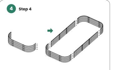
After straight panels are assembled, attach corner panels to straight panels using the same method. Make sure corner panels are attached outside of the straight panels.
