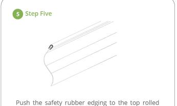
Push the safety rubber edging to the top rolled steel edge and cut the extra length off. Make sure edging is attached securely.
