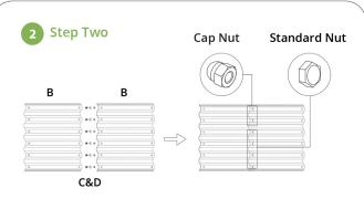
Cap nuts are used for top two rows, standard nuts are used for lower 4 rows. Assemble all straight panels: initially attach all bolts, washers and nuts loosely, and then tighten up using the wrench tool (as supplied) with a screwdriver/cordless drill.
