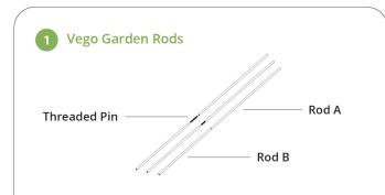
Vego Garden bracing rods are used to reinforce the strength of oversized raised beds. For 2.5ft wide raised bed: use Rod A only; For 4ft wide raised bed: use the Threaded Pin to assemble Rod A & Rod B.
