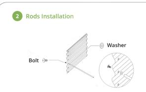
Install the bracing rod between two parallel bolt holes. Attach bolt, panel, washer & rod loosely, in the **4th** bolt hole from the top. Tighten it with the screwdriver for reinforcement of raised bed.
