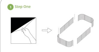
Remove protective films from all panels, and lay panels on a flat surface according to the chosen configuration.
