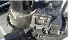
on both sides of the OEM connector behind the bracket, and then pulling the connector out of the hole. Next disconnect the plug from the harness by sliding the tab lock back then pressing the tab and pulling
