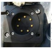
6. Insert and and start each screw a couple turns only, until all are started. Sometimes an awl can help align the holes. Be careful to not cross thread the screws, they should turn fairly easily if properly aligned.
