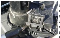
1.Remove the factory connector by depressing the spring clips on both sides of the OEM connector behind the bracket, and then pulling the connector out of the hole. Next disconnect the plug from the harness by sliding the tab lock back
