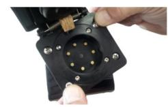
5. Insert the plug with clips attached into the hole at an angle as shown into the OEM hole and then twist clockwise while pressing on the top right and bottom left screws to prevent then from pushing back. The slots in the
