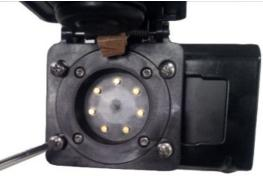
6. Insert the provided wooden block between the index pin and the cover to hold the the cover open. Insert and and start the screws.
