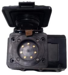
5. Place the new plug into the hole and adjust the clips until the back of the plug sits flush with the bracket.
