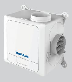
Sentinel Multivent continuous mechanical extract ventilation, MEV is designed for the simultaneous ventilation of separate areas in the home or as a multipoint extraction system for a wide range of commercial applications. The units can be wall, ceiling or loft mounted. Where the ambient air has a high humidity content condensate drains are provided.
