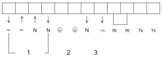
Transmisson:between  $\sim$  and N is always 230V when the transformer handle is in pos. 1-5
