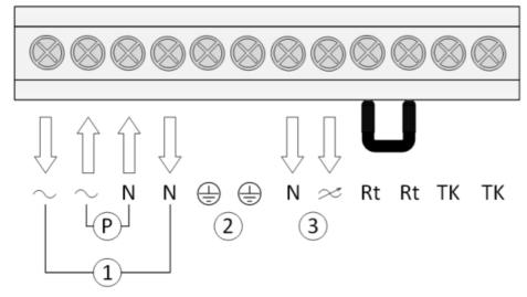
Transmisson:between ~ and N is always 230V when the transformer handle is in pos. 1-5
