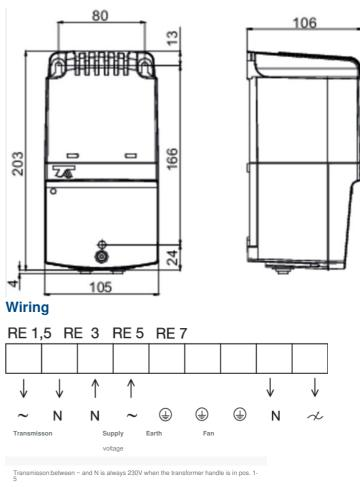
Transmisson:between ~ and N is always 230V when the transformer handle is in pos. 1-5
