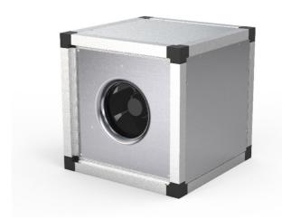
The double skin panels are manufactured from galvanised steel with 30 mm mineral wool insulation. To avoid condensation the profile is provided with a separate chamber to fix screws. The Multibox fans are delivered for straight through airflow but can easily be rebuilt due to removable panels. This allows flexible ventilation solutions. The MUB can also be used as extract- or supply air unit in air handling units. Installation in any mounting position is possible.
