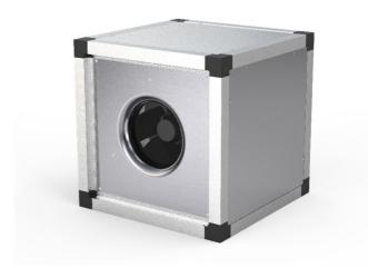
The double skin panels are manufactured from galvanised steel with 30 mm mineral wool insulation. To avoid condensation the profile is provided with a separate chamber to fix screws. The Multibox fans are delivered for straight through airflow but can easily be rebuilt due to removable panels. This allows flexible ventilation solutions. The MUB can also be used as extract- or supply air unit in air handling units. Installation in any mounting position is possible.
