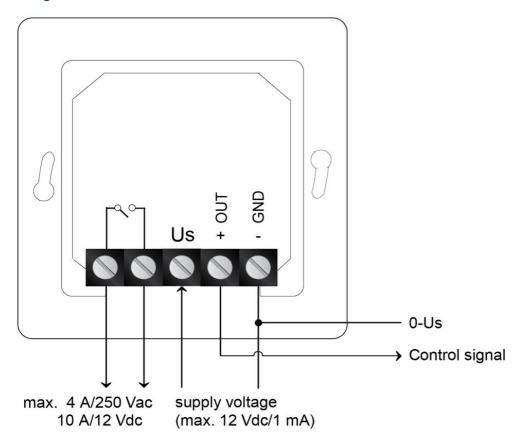
Us = 10V Supply + = 0-10V Output signal - = GND
