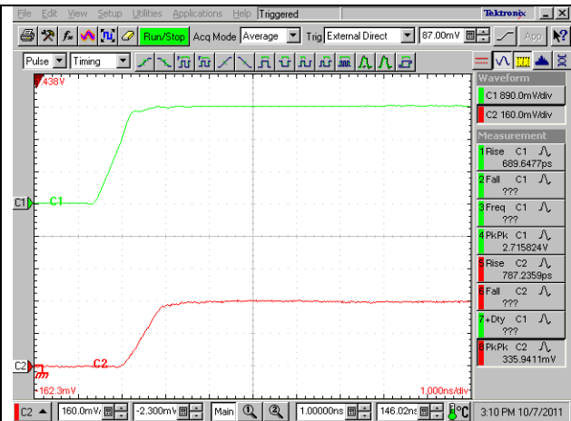
Fig. 9: TDR output waveform with a high quality, wideband 50 \Omega termination
