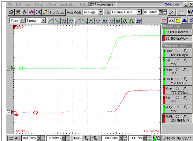
Fig. 12: The incident wave, C2, shows a rise time of 776 ps
