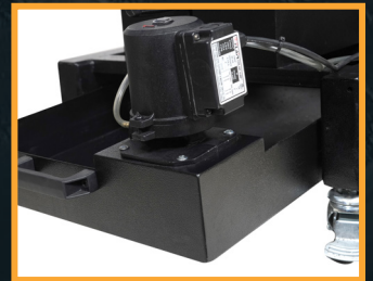
REMOVABLE CHIP TRAY FOR EASY DISPOSAL OF WASTE MATERIAL
