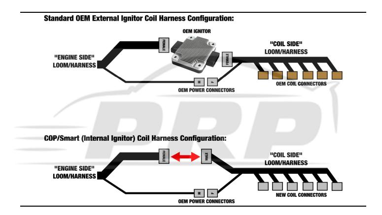
To begin, unplug your current OEM harness. The ends of this harness will be referred to as "Coil Side". The connectors on the other end that are attached to the main engine loom side will be referred to as "Engine Side".
