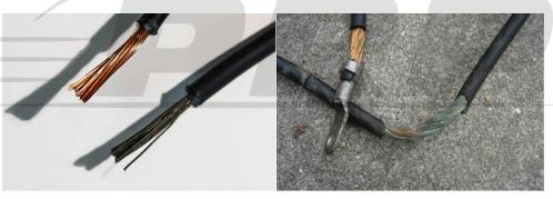
Unfortunately, these wires cannot be repaired, they must be replaced. Not replacing effected wires may result in numerous electrical gremlins (faults) that may seem very intermittent or random and hard to pinpoint.
