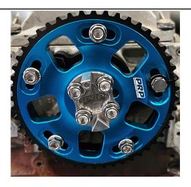
Install the trigger disc on your exhaust cam gear using the M7 bolts provided, (PRP Titanium option pictured). Face the long lug anywhere you like as you will need to set your home signal anyway.
