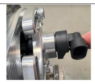
Install the CAS bracket and trigger mount. Also install the black MoTeC sensor. Measure the sensor. The recommended gap for your sensor is 0.4- 1.5 mm off the trigger lug. Use the spacer provided if required.
