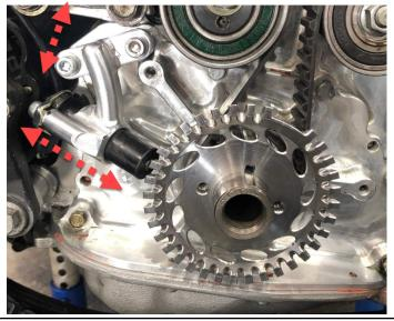
Reinstall the timing belt and new gear/trigger assembly, now you can work on tooth alignment and gap, aim for .050" gap and align the centre trigger sensor pad with the tooth profile by modification of spacing with use of your own initiative.
