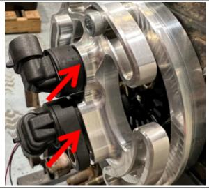
Install the CAS bracket and trigger mount. Also install the black MoTeC sensors. Measure the sensor gaps, you can do this with a feeler gauge under the sensor tabs.
