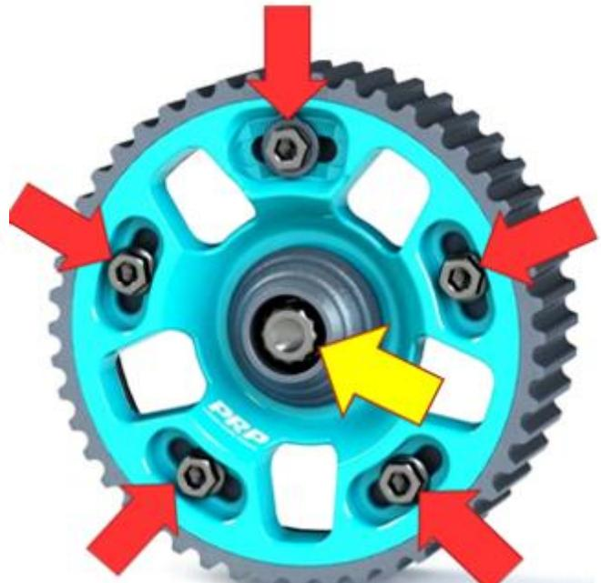
GREEN arrows depicting cam gear M7 RB/CA mounting bolts to torque to 16Nm/11.8 ft Lbs and YELLOW M12 JZ/1UZ/4G63 Cam mount bolt 81 Nm/60 ft Lbs All RED arrows depict cam outer bolts to be tensioned to 14Nm/10.3 ft Lbs. **Note:** same tension for both steel and alloy, the alloy version gear has a longer thread and ti bolt than the steel version.
