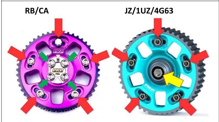
GREEN arrows depicting cam gear M7 RB/CA mounting bolts to torque to 16Nm/11.8 ft Lbs and YELLOW M12 JZ/1UZ/4G63 Cam mount bolt 81 Nm/60 ft Lbs All RED arrows depict cam outer bolts to be tensioned to 14Nm/10.3 ft Lbs. Note: same tension for both steel and alloy, the alloy version gear has a longer thread and ti bolt than the steel version.
