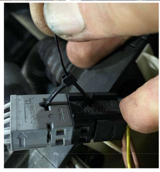
7) Unplug the main green power connector and piggyback the green connectors of the PRP Signal Conversion box into them.
