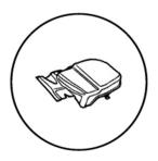
Remove the DME cover, located on the passenger side. Left Hand Drive - Right Side (b).
