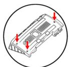
1. Remove Engine Cover, 3 fasteners.
