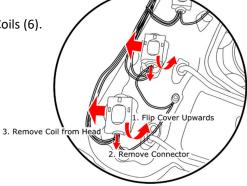
5. Disconnect DME Main Connector and remove coil signal connector.
