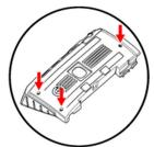
1. Remove Engine Cover, 3 fasteners.
