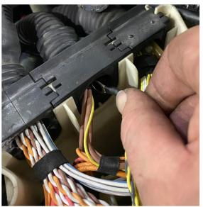
9) Undo chassis ground by strut tower and feed ground through insulation and share the earthing location.
