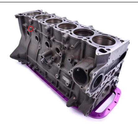
The knock sensor will be installed in this thread located on the rear RHS of the block.
