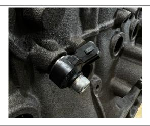
Install the sensor with the 6mm Allen Cap head bolt to 20Nm.
