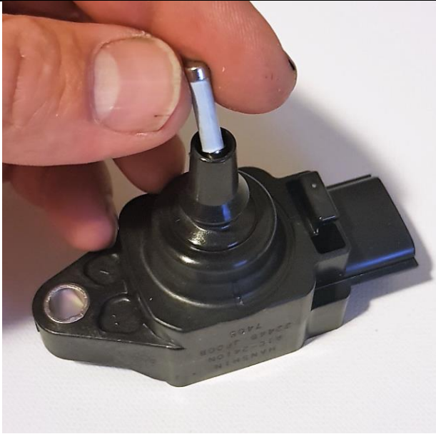
Drop the resistor into the coil head
