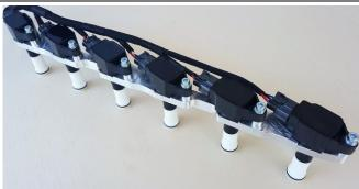
You may now insert the coils, bolt the coil down with the M6 cap bolts, spring and flat washer provided, the coil will seat itself with some downward pressure, you can bolt the bracket down first and insert the coils or put the coils together first and the install the whole kit.
