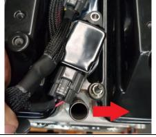
The last modification is to bend this pipe out of the way, use a 3/8 socket extension to give you some leverage.
