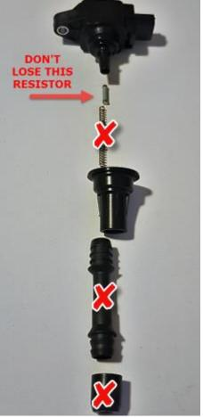
Dissasemble coil and discard these parts
