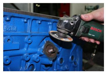
Remove material webbing directly below oil filter area.
