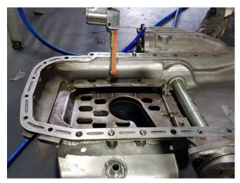
Trial fit your sump to ensure it fits, you may need to clearance a few areas, all sumps are slightly different being cast and we choose to keep as much material in the brace as possible, this area shown above may need a 45 degree linish
