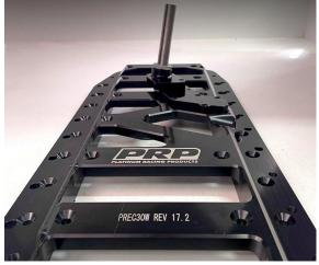
The pipe supplied is made to follow the angle of the sump as it site at 9 degrees, so it makes it easier to fab the pick up square on sump surface (5-8mm off the bottom of the sump is recommended)
