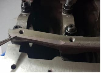
Refief clearance towards the back of the OEM cradle near the 7th main cap is also required as shown.
