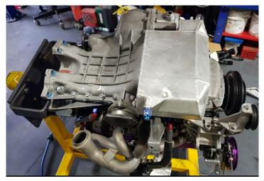
Depending on the sump style / Brand being installed you may need to fit the sump from the bottom so that flaps do not get stuck under your oil pick up.
