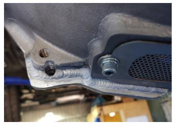
Stencil an addition out of 10mm (or thicker) alloy flat bar, use the gearbox bellhousing to scribe a cut line then cut your shape to match your gearbox, the outer shape can be stenciled against the sump to give a nice meeting surface.
