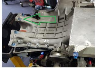
After grinding your welds back flat on the meeting side of the bellhousing, Line the gearbox onto the engine assembly and scribe or use a paint spray can to mark out new bolt hole placement
