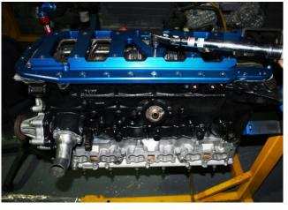
After fitting the oil pick-up you are now ready to bolt the sump on.
