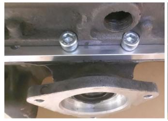
This view shows the bolt relief on the exhaust side of the block using M10 - 1.25x25 bolts.
