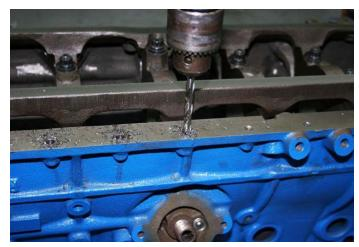
Drill out all original M6 sump bolts with a 6.85mm (17/64) drill or 7.0 mm as shown.
