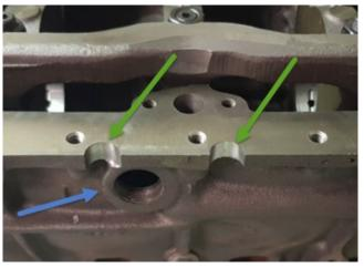
A small section of the turbo oil drain is also to be removed shown here with the blue arrow. This will allow the bolt head to drop through.
