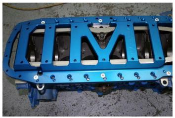
Use at least 4- 6 evenly spaced bolts around the perimiter of the pan rail as shown above to trial fit your brace. Ensure there is no more than 2 thou gap between the PREC and the OEM main cap girdle.
