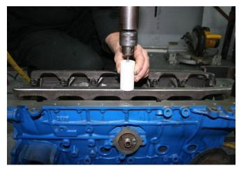
Alternative to the use of a drill press, image above demonstrates the use a drilling guide to assist.
