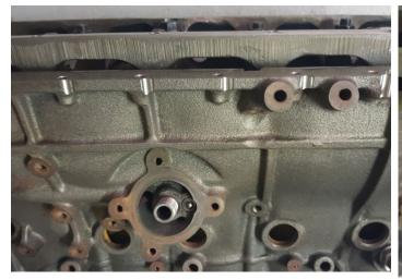
Prepared block should look similar to this on the inlet side of the engine.
