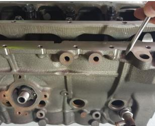
This picture demonstrates the cut out for the rear hole.
