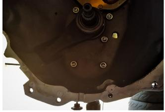
Part the assembly, drill and tap your holes (M10 x 1.5) if using original bolts, you are now ready for assembly.
