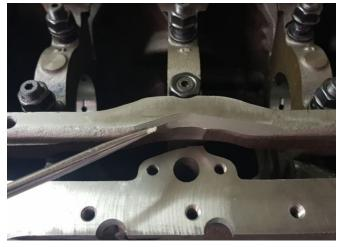
Relieve the OEM cradle near the OEM oil pick up oil gallery to ensure your new wet sump a nice oring seat to seal.
