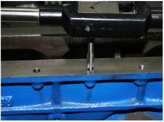
Using an M8 x 1.25 intermediate tap, create new threads as shown.
