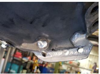
The same can be done for the driver's side, you can choose to weld up the original threaded holes if you wish or leave them, it is inconsequential. Weld the plates on to the bellhousing on both sides, Remember to V out the meeting side for a stronger weld.
