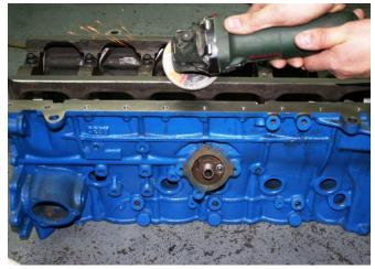
Remove sharp edge of cradle at a 45° angle with a grinder. This will ensure the edge does not come in contact with the inner radius of your PREC.
