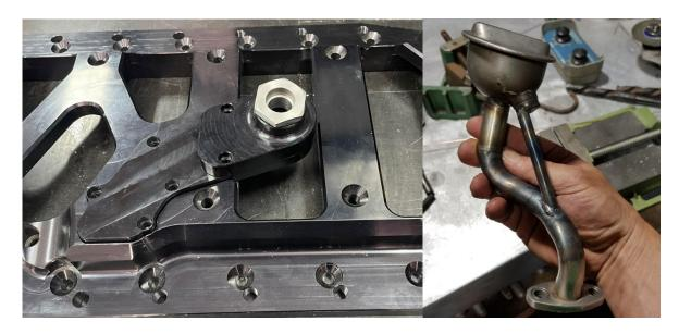
Use the OEM oil pick up or make up your own, cut the OEM oil pick up bowl off and weld it to the pipe provided.
