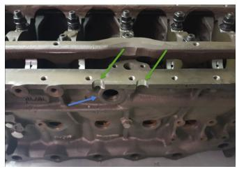
Remove the material on this part of the block as shown with the green arrows. (approx. diameter 16.5mm)
