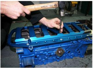
Mark the additional 13 bolt holes through the brace onto the cradle with a centre punch as shown.
