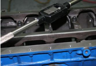
Using an M8 x 1.25 intermediate tap, create new threads into main cap cradle.
