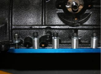
This is view shows the bolt relief on the inlet side of the block using M10 - 1.25x60 bolts fit through assembly with provided tube spacers.
