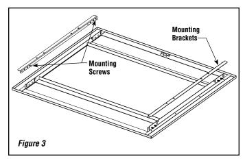
6. Mount both side mounting brackets in the same orientation they were removed from the facade. Plug both upper threaded inserts using provided hardware (six button head screws). See *Figure 4*.
