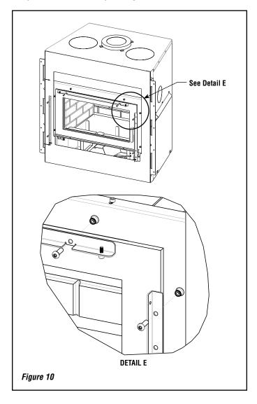
Slide the facade mounting slots onto the four mounting screws located on the top and side mounting brackets and tighten. See Figures 10 and 11.
