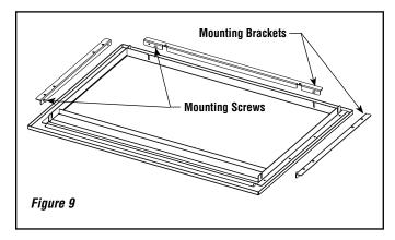
Mount the upper and both side mounting brackets in the same orientation they were removed from the facade, using provided hardware (six button head screws). See Figure 10.
