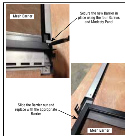
Figure 48B - Barrier Assembly Replacement - Classic Frame
