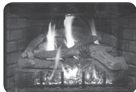
Fig. 52-5 Proper flame appearance
