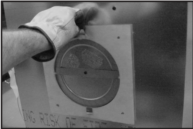
Figure 6.12 (Generic Fireplace Shown) Fold the tabs toward the center of the fire plug (90°) and remove the insulation gasket.
