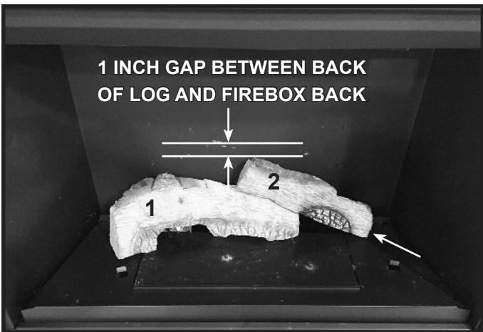
Figure 5. Install Right Rear Base Log
