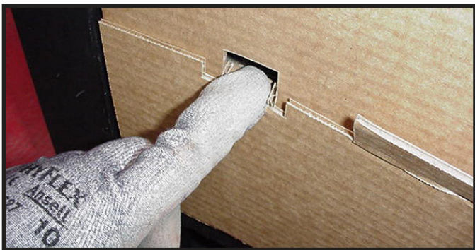
Figure 11.10 Securing Tabs Inside Front of Splatter Guard
