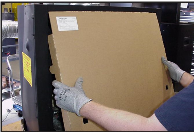
Figure 11.5 Installation of Splatter Guard
