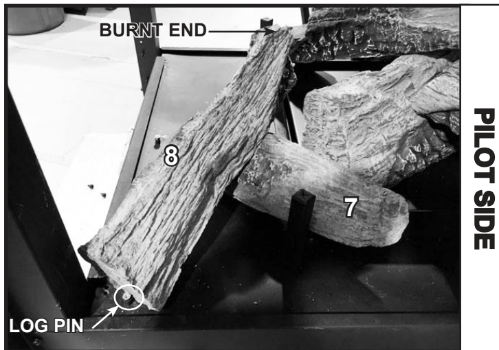
Figure 10. Log #8 Installed
