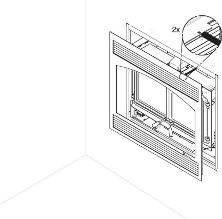
5. Firmly push the faceplate against the fireplace. Using a power driver, secure the bottom with 2 self-tapping screws (one on each side) provided with the fireplace owner's manual.
