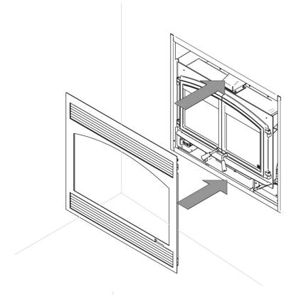
4. Attach the upper springs on the faceplate to hold it in place.
