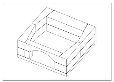
Make a final inspection of all contact joints in the storage base assembly to be sure they are properly sealed.
