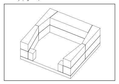
Notch the ends of each sidewall equal to the thickness of the steel as shown. Each end of the steel angles must bear fully at least 3" onto the side wall assembly.
