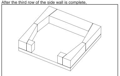
insert 28" rebar vertically through the cells. (Figure 2) Top that off with the fourth row of the storage base.
