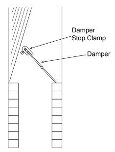
Figure 8 Damper Stop Clamp
