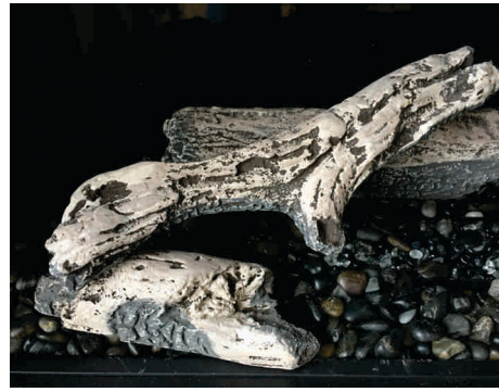
10. Place Left Front Bottom Log (6) under Log 3. Note: This log placement is important in order to raise log 3 up crossing the flame in order to reduce risk of soot.
