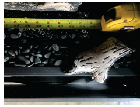
11. Place Far Right Bottom Log (7) as shown taking care to make sure it is not crossing the flame path.
