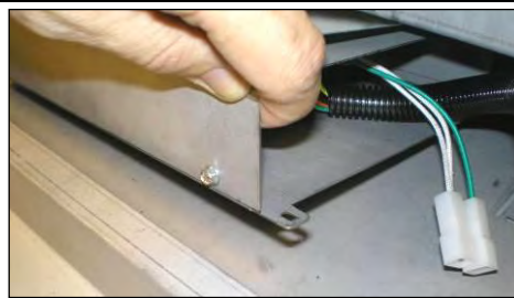
2. Lift UHS Box out of Unit
