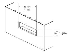
Electrical Connection Requirements: This Appliance ships with a GFCI protected power cord installed. A minimum 15 AMP, 120V/60Hz circuit is required. If hardwiring for an outdoor appliance, the circuit must be Ground Fault Circuit Interrupter (GFCI) Protected.
