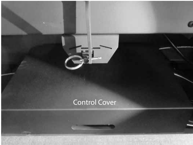
Figure 4.13 Remove Control Cover
