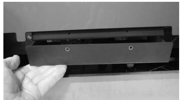
Figure 4.16 Removal of Air Chamber Cover
