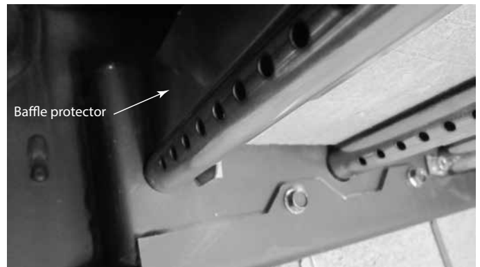
Figure 4.9 Reinstall Baffle Protection Channel
