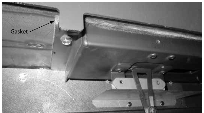
Figure 4.22 Install New Air Chamber
