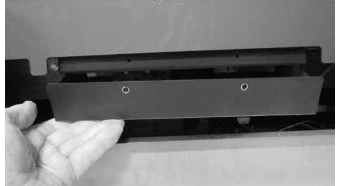
Figure 4.27 Removal of Air Chamber Cover
