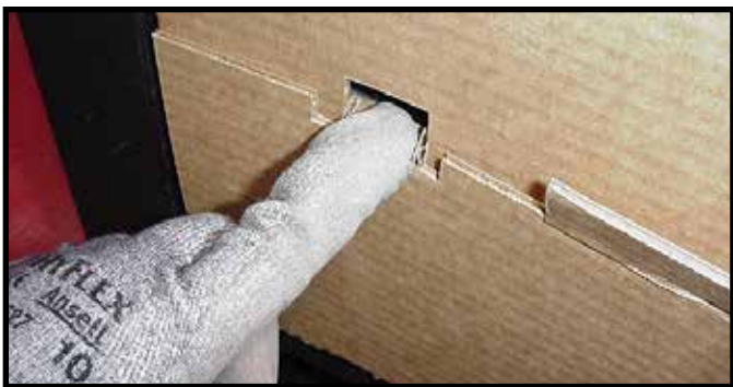
Figure 11.10 Securing Tabs Inside Front of Splatter Guard
