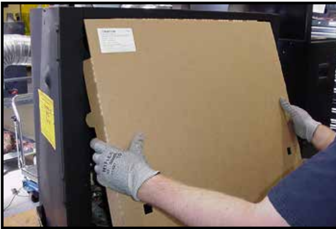
Figure 11.5 Installation of Splatter Guard
