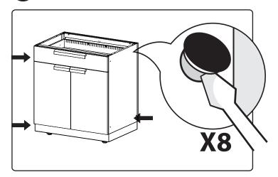
3 Align bolts, tighten lightly.
