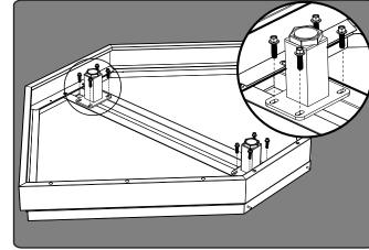
Attach 2 legs to leg channel with 8 x M6 x25mm hex bolts.
