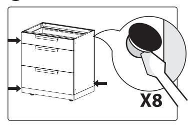
3 Align bolts, tighten lightly.
