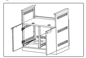
Plip cabinet upside down on protected surface and locate holes on crossbeam.
