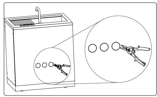
Locate the 3 pre slotted holes in the bottom of the cabinet.
