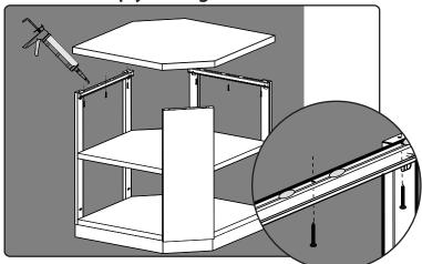
Allow the silicone to dry for 24 hours before loading weight on shelf.
