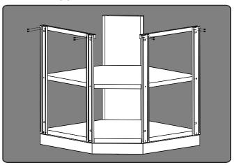
Add silicone using 8 small dabs to hold top in place. Wipe up any extra silicone that seeps out during installation.
