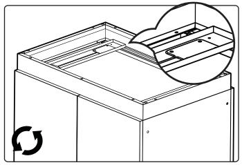
Align foot with holes on crossbeam. Tighten in Hex bolts.
