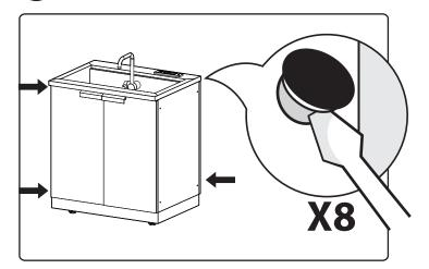
3 Align bolts, tighten lightly.
