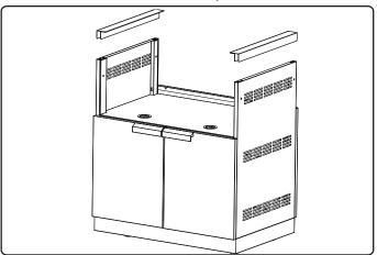
Once the BBQ is centered on the Cart lift up edges of BBQ and Dab a little silicone on the rails to hold it in place
