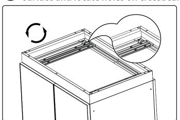
Align caster with holes on crossbeam. Tighten in Hex bolts.
