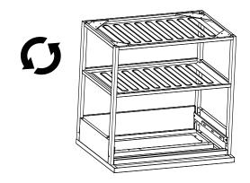
Align foot with holes on crossbeam. Screw in Hex bolts with washer and lock washer.
