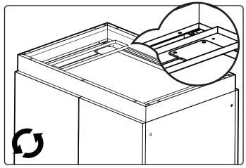
Align foot with holes on crossbeam. Screw in Hex bolts with washer and lock washer.
