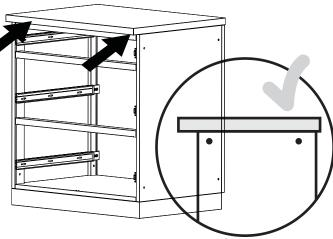
Tighten bolts to secure cabinets.
