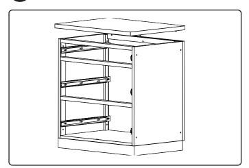
Insert the worktop bolt heads into the keyhole shape slots.
