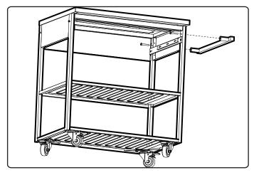
Add Liquor Rail by aligning bolt heads with keyhole slots in tray.
