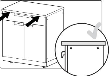
**5** Tighten screws to secure top.
