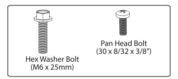
Attach Top, Back Panel and Base with 4 x 8/32" x 3/8" pan head bolts.
