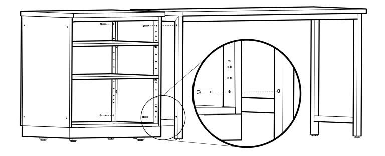
Note: Table has rivet nuts in legs to thread into. Insert bolt from cabinet side.
