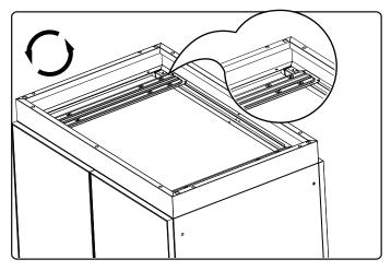
Align foot with rivet nuts on crossbeam. Tighten Hex bolts.
