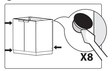
3 Align bolts, tighten lightly.
