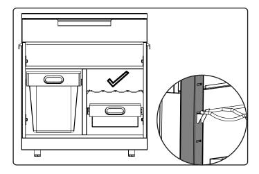
Remove and install beverage chilling tray with formed metal edge.
