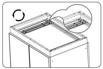
Align leg with rivet nuts on crossbeam. Tighten in Hex bolts . \_\_
