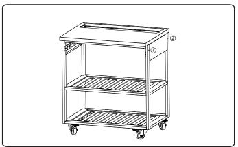
Tighten 2 x 8mm x 60mm bolts. In locations shown here.
