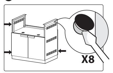
Align bolts, tighten lightly.
