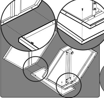
Attach shelf to vertical supports using 4X 8/32" x 3/8" Pan Head Bolts.
