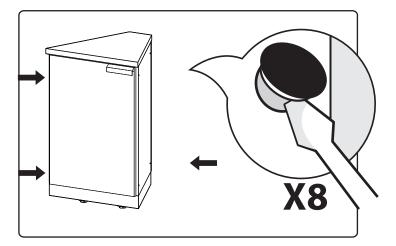
Align bolts, tighten lightly.
