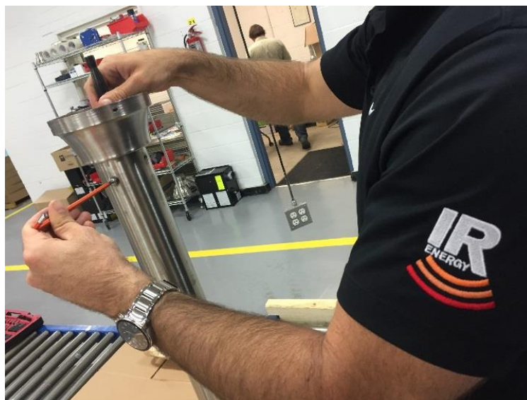
Figure 34: Tighten Pole Neck
