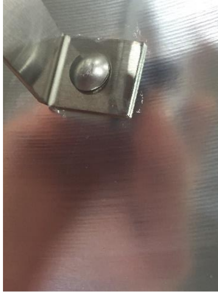
Figure 38: Place Reflector onto Heater Head
