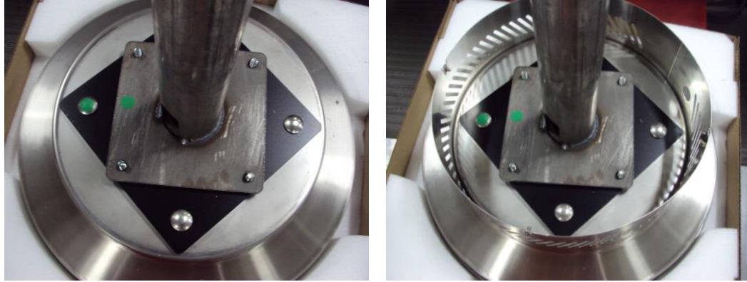
Figure 29: Line Up Pole and Slide Bottom Housing into Place
