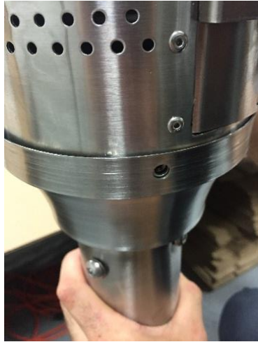
Figure 35: Install Heater Head
