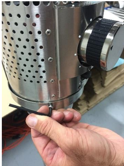
Figure 36: Hand Tighten Heater Head
