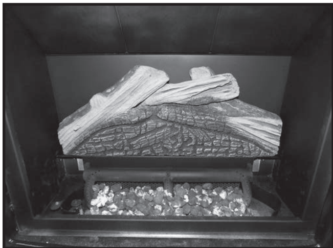
Figure 47: Number 1 log set in place.
