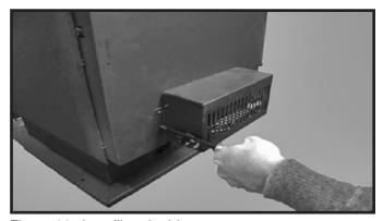
Figure 11: Installing the blower.
