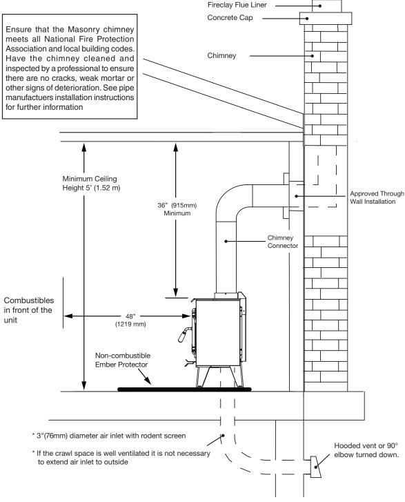
Figure 7: TN10 Venting to a masonry chimney.
