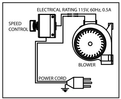
Figure 9: Blower Wiring Diagram.
