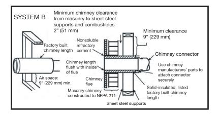
System B. Solid-Insulated, listed factory-built chimney length of the same inside diameter as the chimney connector and having 1 in. (25.4 mm) or more of insulation with a minimum 9 in. (229 mm) air space between the outer wall of the chimney length and combustibles.
