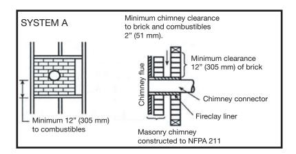
System A. Minimum 3.5 in. (90 mm) thick brick masonry wall framed into combustible wall with a minimum of 12 in. (305 mm) brick separation from clay liner to combustibles. Fireclay liner (ASTM C 315, Standard Specifications for Clay Fire Linings, or equivalent), minimum 5/8 in. (16 mm) wall thickness, shall run from outer surface of brick wall to, but not beyond, the inner surface of chimney flue liner and shall be firmly cemented in place.
