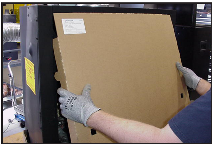
Figure 11.5 Installation of Splatter Guard
