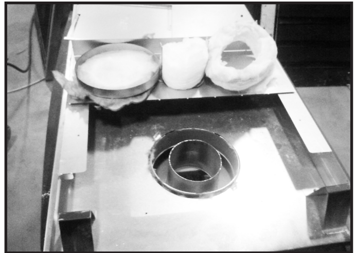
Figure 6.3 Remove and discard the seal cap, insulation donut, insulation plug, and the insulation basket. Attach the first vent section (it will snap into place). Slide the vent gasket onto the vent section and then, up against the appliance. Secure the vent gasket to the appliance with two self-tapping screws found in the manual bag. Note: The vent gasket can be found in the manual bag.
